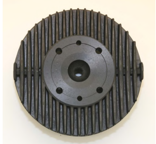
CYLINDER HEAD INTERNAL
